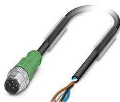
Sensor/actuator cable, 4-position, PUR halogen-free, black-gray RAL 7021, Plug straight M12, coding: A, on free cable end, cable length: 2 m
