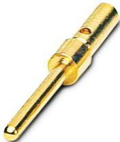
Crimp contact, for D-SUB contact inserts with standard contact density, pin, connection cross section AWG 24 ... 20, punched, gold-plated
