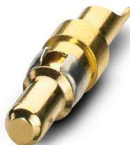
Power contacts, for D-SUB combination inserts, pin, solder cup, straight, rated current 20 A, gold-plated
