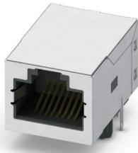
Filtered RJ45 PCB connectors, connection direction of the connector to the PCB: 90 °, Tab up, number of positions: 8, 1 Gbps, THT, Wave, type of packaging: Tray
