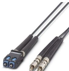
Assembled FO cable, break-out cable, polymer fiber 980/1000 µm, SC-RJ/IP20 on FSMA/IP20, for installation inside the control cabinets, the conductor is suitable for the UV-protected outside insert, length: 1 m
