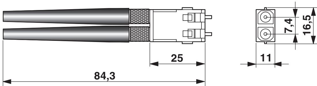
SC-RJ connector, POD, IP20
