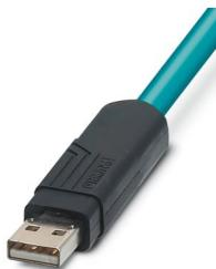
Assembled USB cable, shielded, color: RAL 5021 (water blue), PUR outer sheath, USB type A/standard on open cable end, length: 2 m
