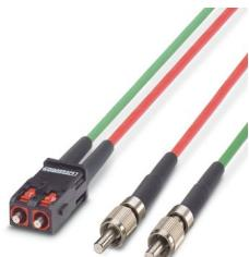
Assembled FO cable, breakout cable, 200/230 µm PCF fiber, SC-RJ/IP20 to FSMA/IP20, for installation inside control cabinets, length: 1 m
