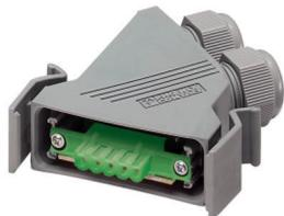
D-SUB connector, degree of protection: IP67, number of positions: 5, material: Plastic, connection method: Screw connection, connection cross section: AWG 24- 12, cable outlet: angled, DeviceNet™
