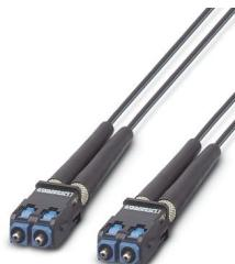
Assembled FO cable, breakout cable, 980/1000 µm polymer fiber, SC-RJ/IP20 to SC-RJ/IP20, for installation inside control cabinets, the cable is suitable for UV-protected outdoor use, length: 2 m
