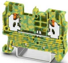
Protective conductor terminal block, number of connections: 2, number of positions: 1, connection method: Push-X-connection, Rated cross section: 1.5 mm<sup>2</sup>, cross section: 0.25 mm<sup>2</sup> - 1.5 mm<sup>2</sup>, mounting type: NS 35/7,5, NS 35/15, color: green-yellow
