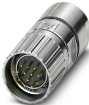
M23, Cable connector, series: M23 PRO, straight, shielded: yes, Screw locking mechanism, No. of pos.: 12, Direction of rotation: Standard, contact connection type: Pin, Crimp connection, cable diameter range: 3 mm ... 15 mm, coding: N, Item is lead-free in accordance with RoHS II without Exemption 6c (Pb < 0.1 %)
