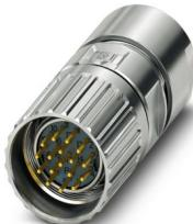
M23, Cable connector, series: M23 PRO, straight, shielded: yes, Screw locking mechanism, No. of pos.: 17, Direction of rotation: Standard, contact connection type: Pin, Crimp connection, cable diameter range: 4 mm ... 8.5 mm, coding: N, Item is lead-free in accordance with RoHS II without Exemption 6c (Pb < 0.1 %)
