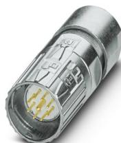
M23, Cable connector, series: M23 PRO, straight, shielded: yes, ONECLICK fast locking system, No. of pos.: 8+1, Direction of rotation: Standard, contact connection type: Pin, Crimp connection, cable diameter range: 3 mm ... 15 mm, coding: N, Item is lead-free in accordance with RoHS II without Exemption 6c (Pb < 0.1 %)
