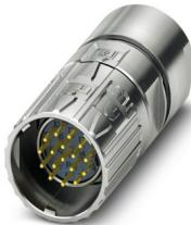
M23, Cable connector, series: M23 PRO, straight, shielded: yes, ONECLICK fast locking system, No. of pos.: 17, Direction of rotation: Standard, contact connection type: Pin, Crimp connection, cable diameter range: 4 mm ... 8.5 mm, coding: N, Item is lead-free in accordance with RoHS II without Exemption 6c (Pb < 0.1 %)
