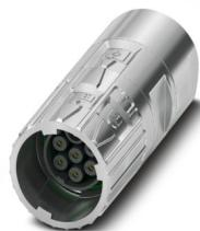
M17, Cable connector, series: M17 PRO, straight, shielded: yes, ONECLICK fast locking system, No. of pos.: 6+PE, contact connection type: Socket, Crimp connection, cable diameter range: 8.5 mm ... 12 mm, Item is lead-free in accordance with RoHS II without Exemption 6c (Pb < 0.1 %)
