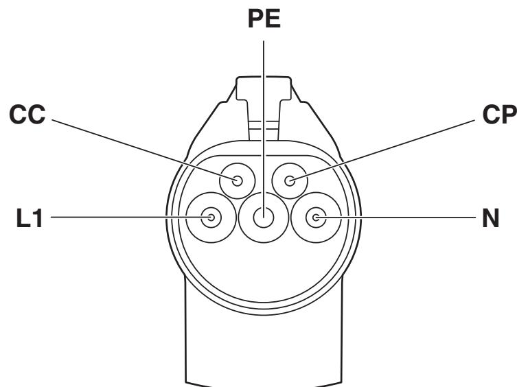
Pin assignment of the Vehicle Connector
