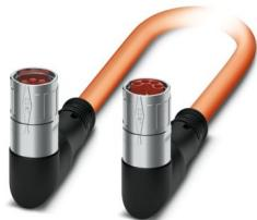
Connector in molded plastic on both sides, series: KSH, M23-Socket, angled rotatable, -120° left/120° right, number of positions: 4+4+4+PE, type of locking: SPEEDCON, on M23-Pin, angled rotatable, -120° left/120° right, number of positions: 4+4+4+PE, type of locking: SPEEDCON, cable length: 15 m, shielded: yes, color of outer sheath: orange RAL 2003
