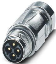
Coupler connector, straight, for standard and SPEEDCON interlock, M17, number of positions: 3+PE, contact connection type: Pin, shielded: yes, degree of protection: IP67, cable diameter range: 10 mm ... 12.5 mm, number of positions: 4, connection method: Crimp connection, series: ST, This product is in the process of being discontinued. This product must no longer be considered for new projects. Please contact your sales representative for alternatives.
