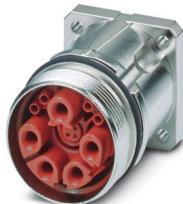
M40, Device connector front mounting, series: SB, straight, shielded: yes, for standard and SPEEDCON interlock, No. of pos.: 8+4+PE, contact connection type: Socket, Crimp connection, Axial O-ring, flange dimensions: 40 mm x 40 mm, coding: Signal, coding 1, this item is expected to be lead-free from Q2 2026 in accordance with RoHS II without exception 6c (Pb < 0.1%), a lead-free alternative is possible on request in advance
