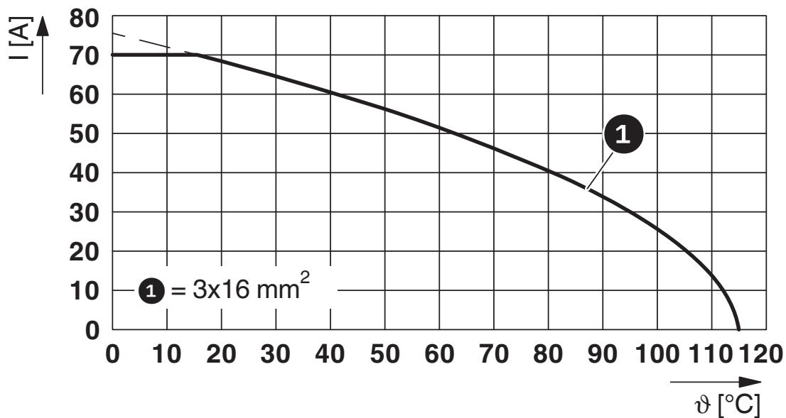
$I$  = current strength,  $\vartheta$  = ambient temperature, power contacts A–C: 3x up to 70 A, signal contacts: 4x 2 A constant, data contacts: no load
