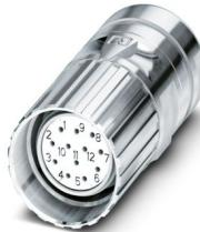
M23, Cable connector, series: CA, straight, shielded: yes, Screw locking mechanism, No. of pos.: 12, Direction of rotation: Counter direction, contact connection type: Pin, Solder connection, cable diameter range: 6 mm ... 10 mm, coding: N
