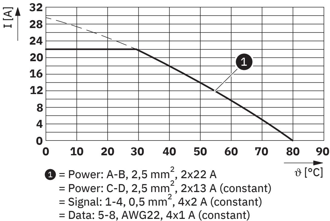
$I$  = current strength,  $\vartheta$  = ambient temperature, power contacts A-B:  $2.5 \text{ mm}^2$ ,  $2 \times 22 \text{ A}$ , power contacts C-D:  $2.5 \text{ mm}^2$ ,  $2 \times 13 \text{ A}$  (constant), signal contacts 1-4:  $0.5 \text{ mm}^2$ ,  $4 \times 2 \text{ A}$  (constant), data contacts 5-8: AWG22,  $4 \times 1 \text{ A}$  (constant)
