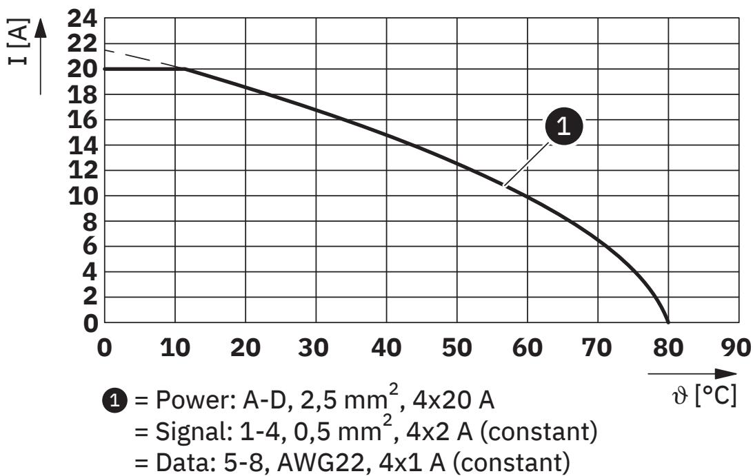
$I$  = current strength,  $\vartheta$  = ambient temperature, power contacts A-D: 2.5 mm<sup>2</sup>, 4 x 20 A, signal contacts 1-4: 0.5 mm<sup>2</sup>, 4 x 2 A (constant), data contacts 5-8: AWG22, 4 x 1 A (constant)
