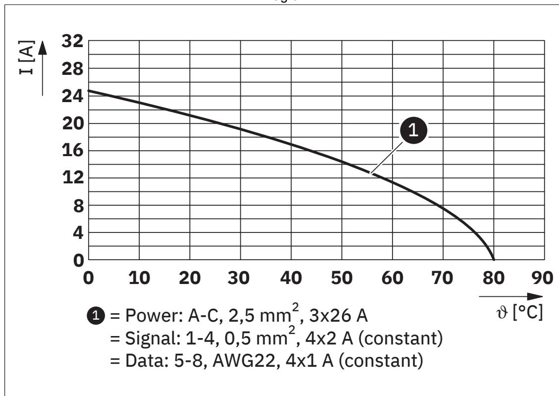
$I$  = current strength,  $\vartheta$  = ambient temperature, power contacts A-C:  $2.5 \text{ mm}^2$ ,  $3 \times 36 \text{ A}$ , signal contacts 1-4:  $0.5 \text{ mm}^2$ ,  $4 \times 2 \text{ A}$  (constant), data contacts 5-8: AWG22,  $4 \times 1 \text{ A}$  (constant)
