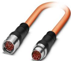
Connector in molded plastic on both sides, series: KSH, M23-Socket, Straight, plastic molded, number of positions: 4+4+4+PE, type of locking: SPEEDCON, on M23-Pin, Straight, plastic molded, number of positions: 4+4+4+PE, type of locking: SPEEDCON, cable length: 2 m, shielded: yes, color of outer sheath: orange RAL 2003, this item is expected to be lead-free from Q2 2026 in accordance with RoHS II without exception 6c (Pb < 0.1%), a lead-free alternative is possible on request in advance
