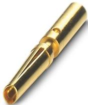
Crimp contact, Socket, turned, contact diameter: 0.8 mm, connection cross section: 0.34 mm<sup>2</sup> ... 0.5 mm<sup>2</sup>, contact material: CuZn, Alternative product in accordance with RoHS II without Exemption 6c (Pb < 0.1 %) item no.: 1244457
