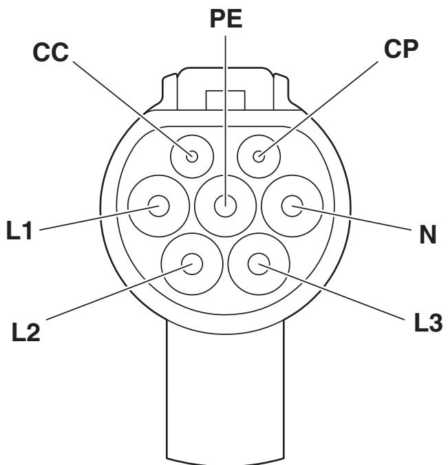
Pin assignment of the Vehicle Connector
