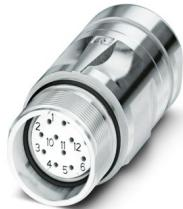
M23, Coupler connector, series: CA, straight, shielded: yes, for standard and SPEEDCON interlock, No. of pos.: 12, Direction of rotation: Standard, contact connection type: Socket, Crimp connection, cable diameter range: 3 mm ... 14.5 mm, coding: N. This product is in the process of being discontinued. This product must no longer be considered for new projects. Please contact your sales representative for alternatives.
