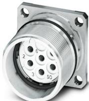
M23, Device connector front mounting, series: CA, straight, shielded: yes, for standard and SPEEDCON interlock, No. of pos.: 8+1, Direction of rotation: Standard, contact connection type: Socket, Solder connection, Flat gasket, flange dimensions: 25 mm x 25 mm, coding: N. This product is in the process of being discontinued. This product must no longer be considered for new projects. Please contact your sales representative for alternatives.
