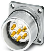
M23, Device connector front mounting, series: CA, straight, shielded: yes, for standard and SPEEDCON interlock, No. of pos.: 8+1, Direction of rotation: Standard, contact connection type: Pin, Crimp connection, Flat gasket, flange dimensions: 25 mm x 25 mm, coding: N. This product is in the process of being discontinued. This product must no longer be considered for new projects. Please contact your sales representative for alternatives.
