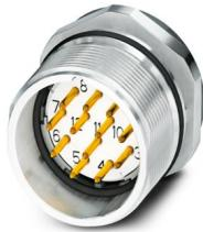
M23, Device connector front mounting, series: CA, straight, shielded: yes, for standard and SPEEDCON interlock, No. of pos.: 12, Direction of rotation: Standard, contact connection type: Pin, Crimp connection, Axial seal, coding: N. This product is in the process of being discontinued. This product must no longer be considered for new projects. Please contact your sales representative for alternatives.
