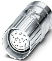
M23, Cable connector, series: CA, straight, shielded: yes, Screw locking mechanism, No. of pos.: 12, Direction of rotation: Standard, contact connection type: Socket, Crimp connection, cable diameter range: 6 mm ... 10 mm, coding: N. This product is in the process of being discontinued. This product must no longer be considered for new projects. Please contact your sales representative for alternatives.
