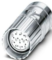
M23, Cable connector, series: CA, straight, shielded: yes, Screw locking mechanism, No. of pos.: 17, Direction of rotation: Standard, contact connection type: Socket, Solder connection, cable diameter range: 6 mm ... 10 mm, coding: N. This product is in the process of being discontinued. This product must no longer be considered for new projects. Please contact your sales representative for alternatives.
