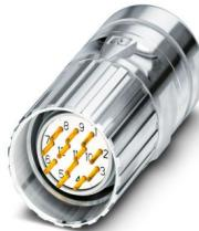
M23, Cable connector, series: CA, straight, shielded: yes, Screw locking mechanism, No. of pos.: 17, Direction of rotation: Standard, contact connection type: Pin, Crimp connection, cable diameter range: 6 mm ... 10 mm, coding: N. This product is in the process of being discontinued. This product must no longer be considered for new projects. Please contact your sales representative for alternatives.
