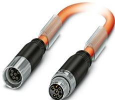
Connector in molded plastic on both sides, series: KST, M17-Socket, Straight, plastic molded, number of positions: 5+PE, type of locking: Screw locking mechanism, on M17-Pin, Straight, plastic molded, number of positions: 5+PE, cable length: 10 m, shielded: yes, color of outer sheath: orange RAL 2003, this item is expected to be lead-free from Q1 2027 in accordance with RoHS II without exception 6c (Pb < 0.1%), a lead-free alternative is possible on request in advance
