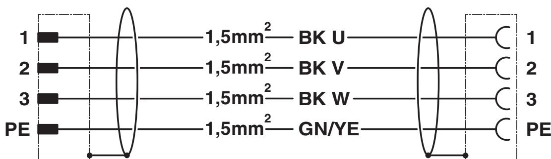
Contact assignment of M17 plugs/sockets, cable type B00
