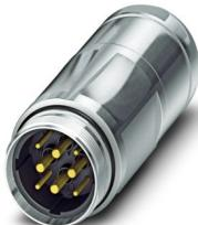
Coupler connector, straight, for standard and SPEEDCON interlock, M40, number of positions: 4+3+PE, contact connection type: Pin, shielded: yes, degree of protection: IP67, cable diameter range: 20.5 mm ... 26.5 mm, number of positions: 8, connection method: Crimp connection, series: SM, this item is expected to be lead-free from Q4 2025 in accordance with RoHS II without exception 6c (Pb < 0.1%), a lead-free alternative is possible on request in advance
