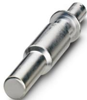
Crimp contact, Pin, turned, contact diameter: 10 mm, connection cross section: 10 mm<sup>2</sup> ... 10 mm<sup>2</sup>, contact material: CuZn, Alternative product in accordance with RoHS II without Exemption 6c (Pb < 0.1 %) item no.: 1362824
