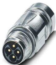
Coupler connector, straight, for standard and SPEEDCON interlock, M17, number of positions: 3+PE, contact connection type: Pin, shielded: yes, degree of protection: IP67, cable diameter range: 5 mm ... 8 mm, number of positions: 4, connection method: Crimp connection, series: ST, This product is in the process of being discontinued. This product must no longer be considered for new projects. Please contact your sales representative for alternatives.
