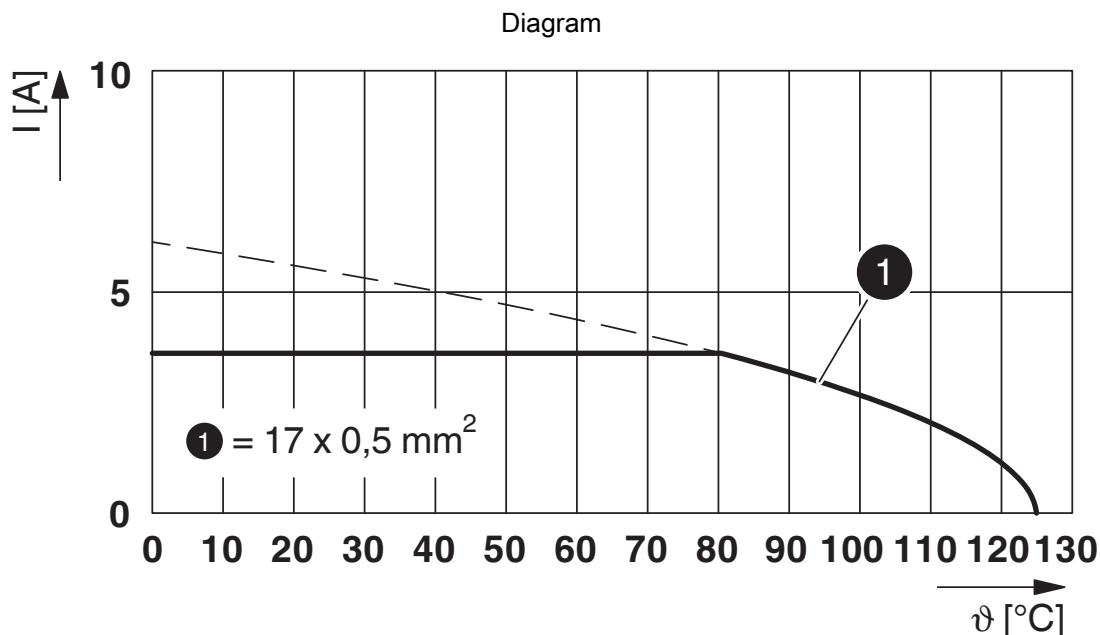
$I$  = current strength,  $\vartheta$  = ambient temperature,  $17 \times 3.6 \text{ A}$
