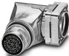
Device connector front mounting, angled rotatable, SPEEDCON, M17, number of positions: 17, contact connection type: Pin, Axial O-ring, shielded: yes, flange dimensions: 21.6 mm x 21.6 mm, degree of protection: IP67, number of positions: 17, connection method: Crimp connection, series: ST, This product is in the process of being discontinued. This product must no longer be considered for new projects. Please contact your sales representative for alternatives.
