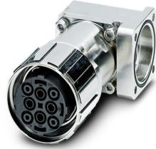
Device connector front mounting with knurled nut, angled fixed, Screw locking mechanism, M40, number of positions: 2+3+PE, contact connection type: Socket, Axial O-ring, shielded: yes, flange dimensions: 40 mm x 40 mm, number of positions: 6, connection method: Crimp connection, series: SM, this item is expected to be lead-free from Q3 2026 in accordance with RoHS II without exception 6c (Pb < 0.1%), a lead-free alternative is possible on request in advance
