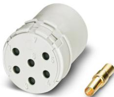
Contact insert, M23, number of positions: 6, contact connection type: Socket, Crimp connection, series: NC, RC, RM, TU, UC, this item is expected to be lead-free from Q4 2025 in accordance with RoHS II without exception 6c (Pb < 0.1%), a lead-free alternative is possible on request in advance
