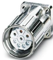
Device connector front mounting with knurled nut, straight, Screw locking mechanism, M23, number of positions: 4+3+PE, contact connection type: Socket, Axial O-ring, shielded: yes, flange dimensions: 26 mm x 26 mm, cable diameter range: 0 mm ... 0 mm, number of positions: 8, connection method: Crimp connection, series: SF, This product is in the process of being discontinued. This product must no longer be considered for new projects. Please contact your sales representative for alternatives.
