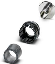
Cable clamp type cage and shield adapter, shielded: yes, litz wire bundle diameter: 5.5 mm, cable diameter range: 7.5 mm ... 9.5 mm, series: NC, RC, this item is expected to be lead-free from Q4 2025 in accordance with RoHS II without exception 6c (Pb < 0.1%), a lead-free alternative is possible on request in advance
