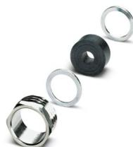
Cable gland, material for screw connection: Brass, nickel-plated, external cable diameter 4 mm .. . 14 mm, shielding: no, connecting thread: M20 x 1.5, series: RM
