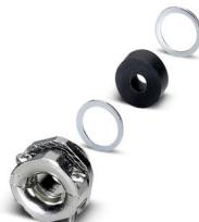
Cable gland, material for screw connection: Brass, nickel-plated, external cable diameter 7 mm .. . 10 mm, shielding: no, connecting thread: Pg9, series: RC, this item is expected to be lead-free from Q4 2025 in accordance with RoHS II without exception 6c (Pb < 0.1%), a lead-free alternative is possible on request in advance
