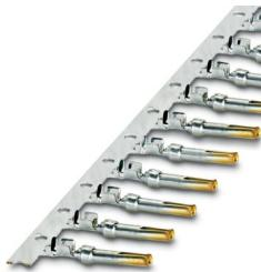
Crimp contact, Socket, rolled, contact diameter: 1 mm, connection cross section: 0.22 mm<sup>2</sup> ... 0.56 mm<sup>2</sup>, contact material: Cu alloy, Taped product, 500 pcs. per ribbon, Item is lead-free in accordance with RoHS II without Exemption 6c (Pb < 0.1 %)
