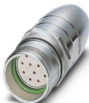
M23, Coupler connector, series: RC, straight, shielded: yes, Screw locking mechanism, No. of pos.: 17, Direction of rotation: Standard, contact connection type: Socket, Solder cup, cable diameter range: 7.5 mm ... 9.5 mm, coding: N
