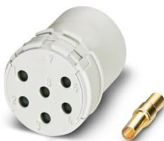
Contact insert, M23, number of positions: 12, contact connection type: Socket, Crimp connection, series: NC, RC, RM, TU, UC, this item is expected to be lead-free from Q4 2025 in accordance with RoHS II without exception 6c (Pb < 0.1%), a lead-free alternative is possible on request in advance
