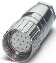
M23, Cable connector, series: RC, straight, shielded: no, Screw locking mechanism, No. of pos.: 12, Direction of rotation: Standard, contact connection type: Socket, Solder cup, coding: N. This product is in the process of being discontinued. This product must no longer be considered for new projects. Please contact your sales representative for alternatives.
