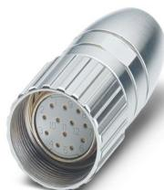
M23, Cable connector, straight, Screw locking mechanism, No. of pos.: 8+1, Direction of rotation: Standard, contact connection type: Socket, Crimp connection, cable diameter range: 7.5 mm ... 9.5 mm, coding: N
