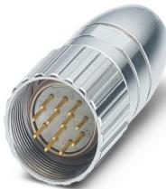
M23, Cable connector, straight, Screw locking mechanism, No. of pos.: 8+1, Direction of rotation: Standard, contact connection type: Pin, Solder cup, cable diameter range: 5.5 mm ... 6.5 mm, coding: N
