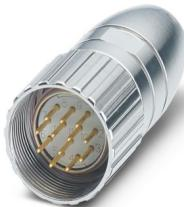
M23, Cable connector, straight, Screw locking mechanism, No. of pos.: 8+1, Direction of rotation: Standard, contact connection type: Pin, Solder cup, cable diameter range: 6.5 mm ... 7.5 mm, coding: N. This product is in the process of being discontinued. This product must no longer be considered for new projects. Please contact your sales representative for alternatives.
